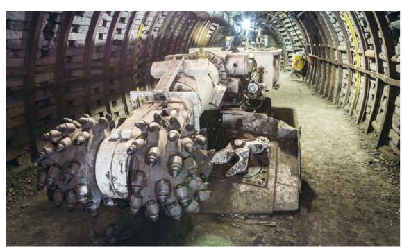
Continuous heading machine for tunnelling
